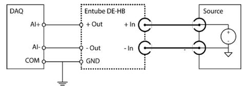
The schematic on the figure above shows how to connect the Enforce HS between the input signal source and the data acquisition.
