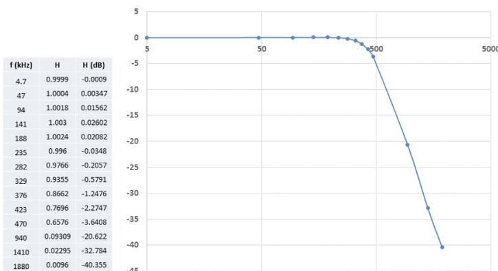
0.05% deviation at 50kHz, 0.5% deviation at 250kHz, -3dB at 450kHz, -22dB at 1MHz
